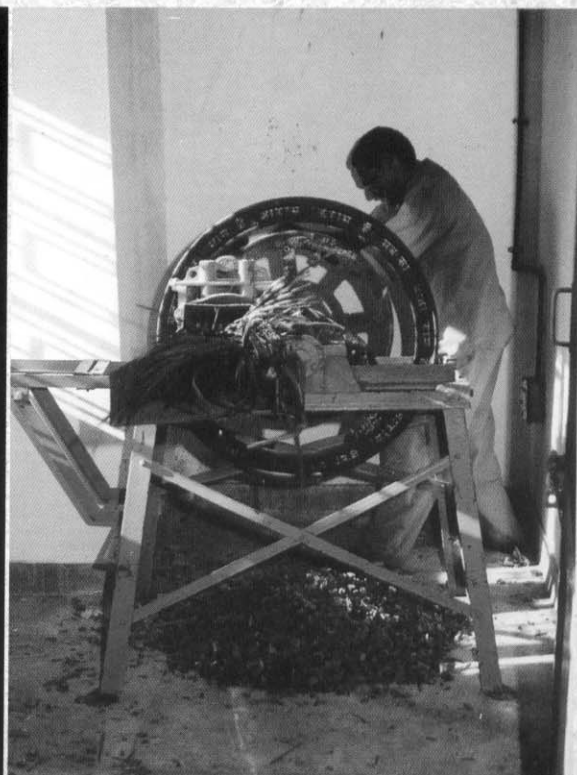
Chaff cutter for cutting coconut wastes
