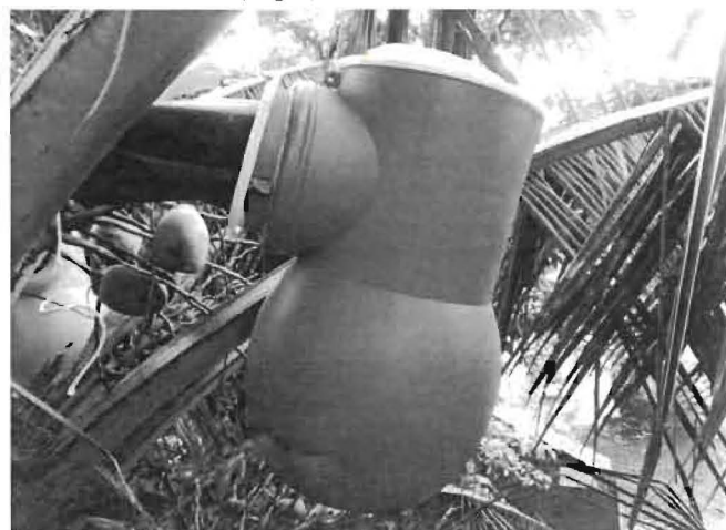
Fig. 5: Coco-sap chiller developed by ICAR-CPCRI for the collection of unfermented coconut inflorescence sap.
