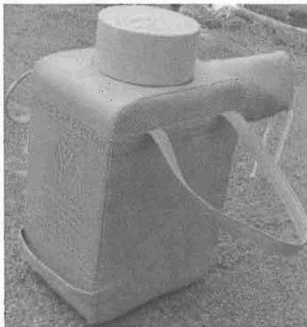
Fig. 13: Coco sap chiller
