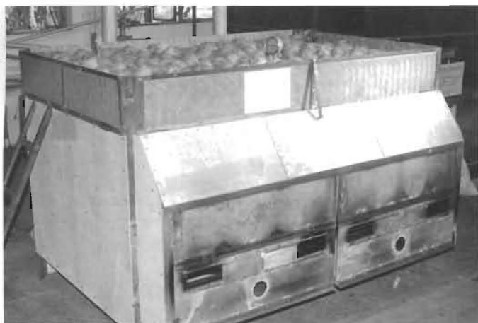
Shell fired copra dryer
