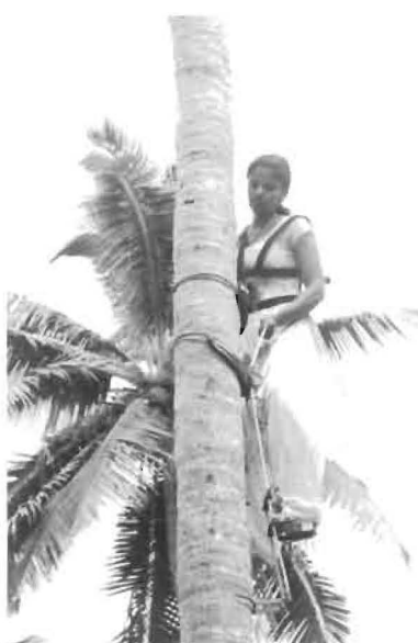
Chemberi model of coconut climbing machine
