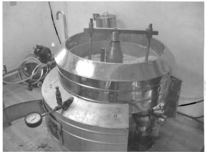
Agricultural waste fired virgin coconut oil cooker
