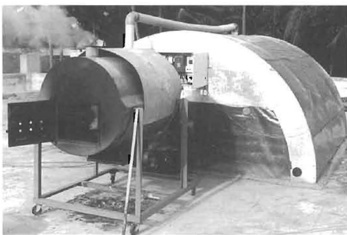
Solar-cum-electrical dryer with agricultural waste as third source of energy
