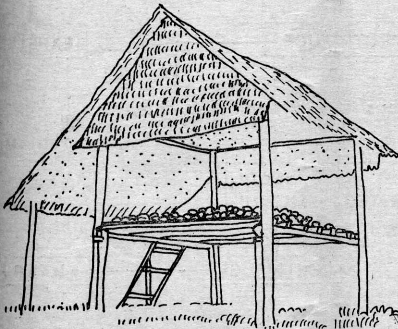
Fig. 2. A primitive copra kiln, or smoke house offering protection from the rain.
