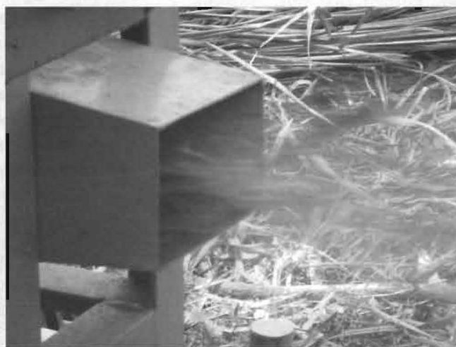
Chaffed material from shredder outlet
