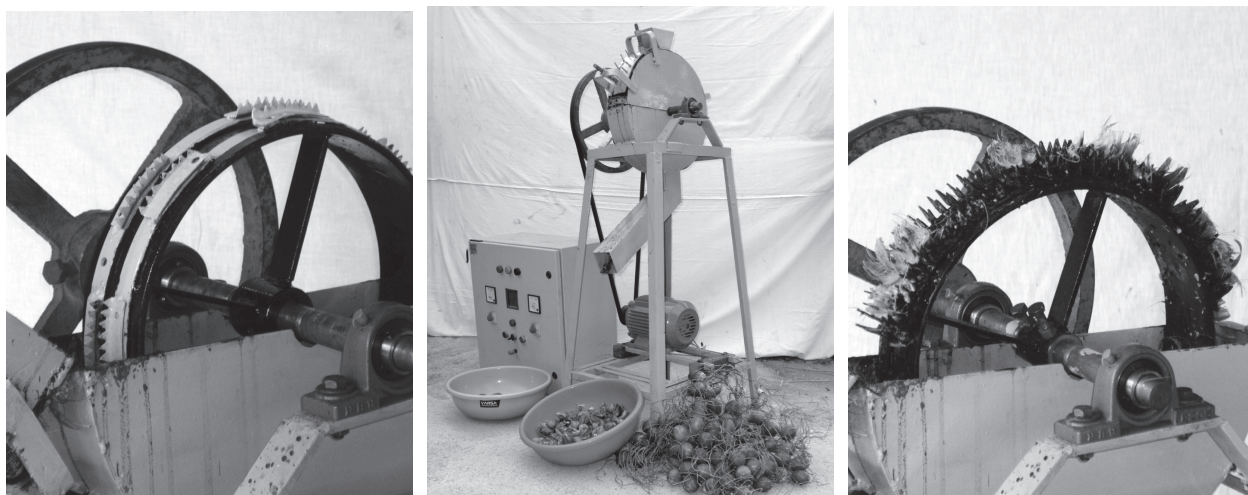
Fig. 6. Arecanut dehusker with different types of dehusking rotors
