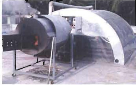
Fig. 2.50: Solar cum electrical dryer with agricultural waste as third source of energy
