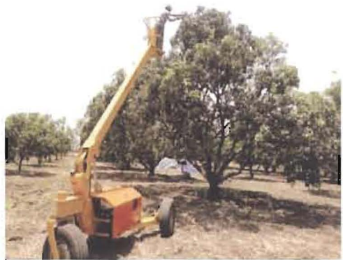
Fig. 2.36: A view of harvesting of mango using CIAE developed self-propelled hydraulic multipurpose system
