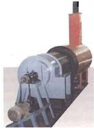
Fig. 2.48: Forced circulation copra dryer
