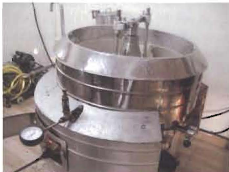
Fig. 2.73: Agricultural Waste Fired Virgin Coconut Oil Cooker
