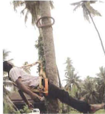
Fig. 2.41: CPCRI safety attachment for traditional coconut climbing
