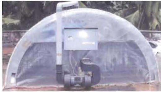
Fig. 2.49: Solar tunnel dryer with electricity as an alternate source of energy
