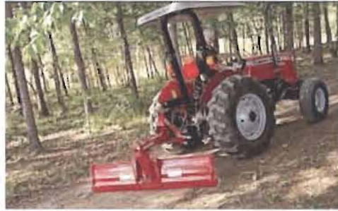
Fig.2.3: Tractor Mounted Terracer Blade (Source- http://www.agro-implements.com/terracer-blade-land-leveller.html accessed on 19.03.2016)
