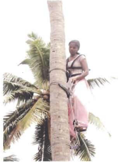
Fig. 2.38: Chemberi model coconut climbing machine
