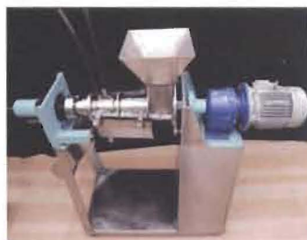
Fig. 2.71: Single Screw Type Coconut Milk Expeller with cooling mechanism
