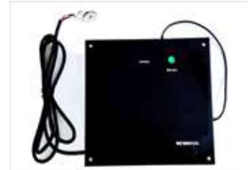
Acoustics based red palm weevil detector
