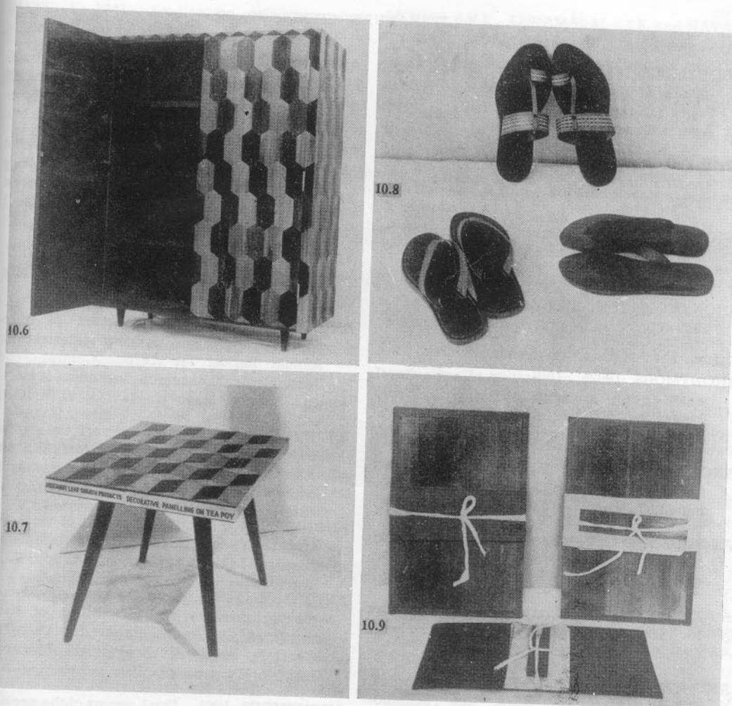
Figs. 10.6—10.9 Useful items made out of areca leaf sheath. Fig. 10.6—10.7 Decorative panels of wooden almirah and teapoy; Fig. 10.8 Chappals and sandals with areca leaf sheath sole tops; Fig. 10.9 File boards and flaps made out of areca leaf sheath.
