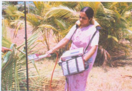
Fig. 3 : Portable photosynthesis system (LCA-4) measures both \text{CO}_2 fixation and \text{H}_2\text{O} transpired. Note the leaflet clipped to the chamber held with the right hand. The values are displayed on the screen.
