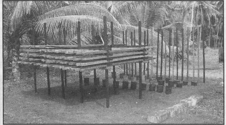
Timber kept exposed with ground contact and without ground contact
