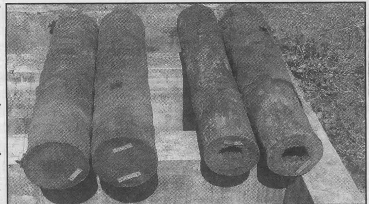
Left - Timber without treatment. Right - Timber treated with wood preservative creosote
