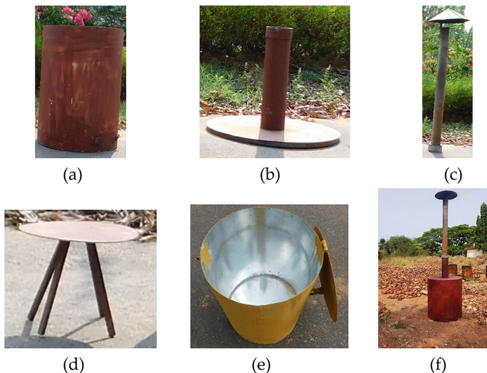
Fig. 1 Components of pyrolysis unit used for production of biochar from tender coconut husk. a Combustion chamber. b Lid for combustion chamber. c Exhaust pipe. d Stand of pyrolysis tank. e Pyrolysis (inner) chamber. f biochar production setup
