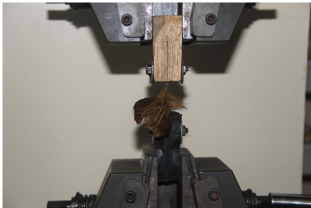
Fig. 5a. Measurement of detachment force for bunch of fibres separation.
