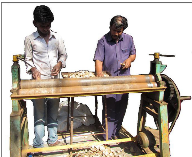
Fig. 2a. Pressing of arecanut husk in sheet bending setup.
