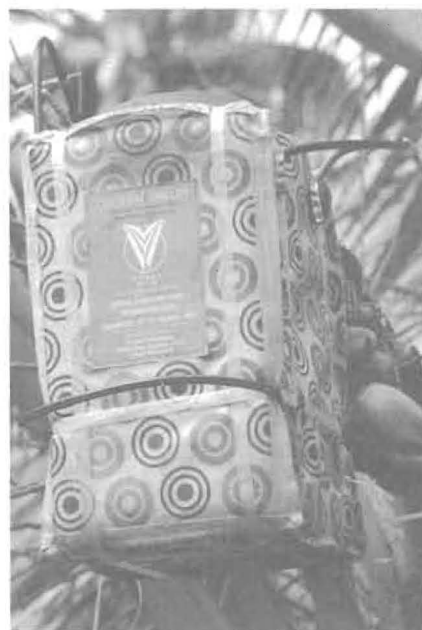
Figure 5. 'Coco-sap chiller' developed by CPCRI for the collection of hygienic and unfermented sap.
