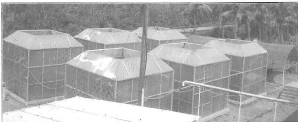
Figure 2.3: Open Top Chamber Facility for Studying the Effect of Elevated CO 2 and Temperature at CPCRI, Kasaragod, India.
