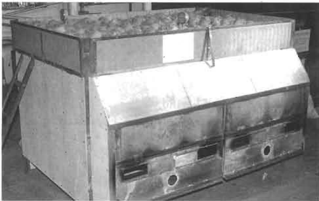
Shell Fired Copra Dryer
