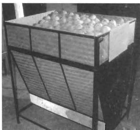
Waste fired copra dryer
