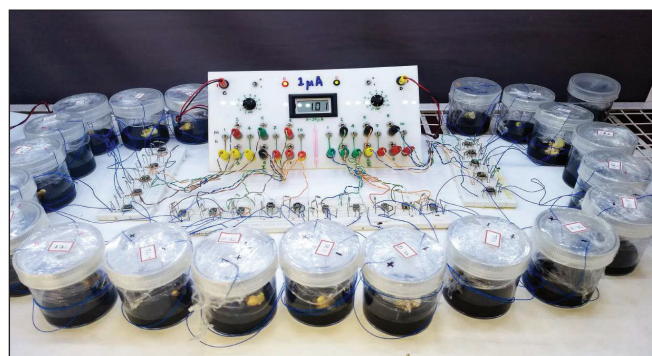
Figure 5: Experiment setup – 1 \mu\text{A} for 20 channels
