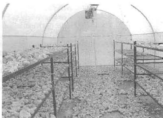
Fig. 1—Drying of copra inside solar tunnel drier
