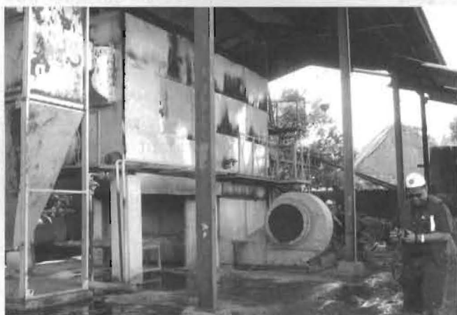
Manufacture of shell charcoal through waste heat method: Heat generated is the major source energy for the DC industry
