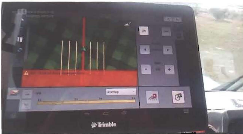
Figure 2 The setup of GPS guidance system of autopilot mode for tracking the straight-line routes in the field
