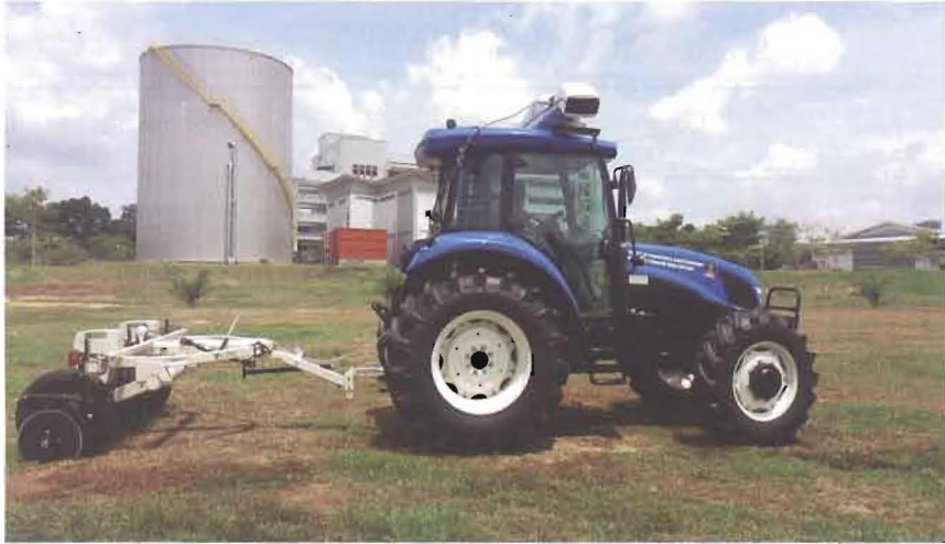
Figure 1 The autopilot tractor used in this study with nitrogen-sensor on the top of cab and soil EC sensor on the back
