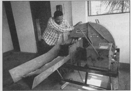
4. Arecaleaf sheath cutting machine in operation
