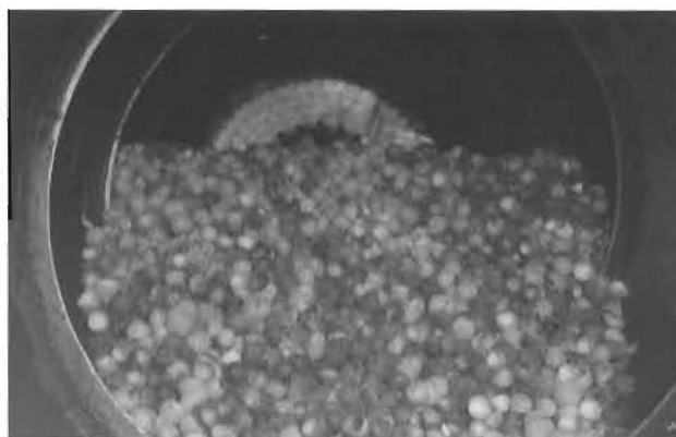
Fig.2 Coconut Shell inside the Rotating Reactor
