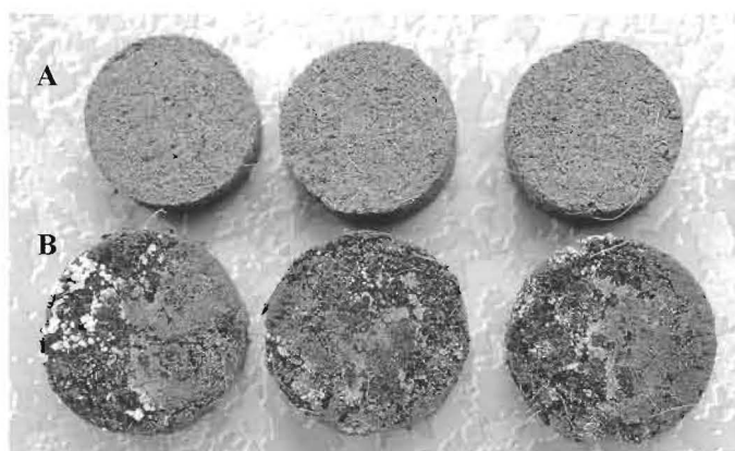
Trichoderma enriched coir pith cake before activation (A) and after activation (B)
