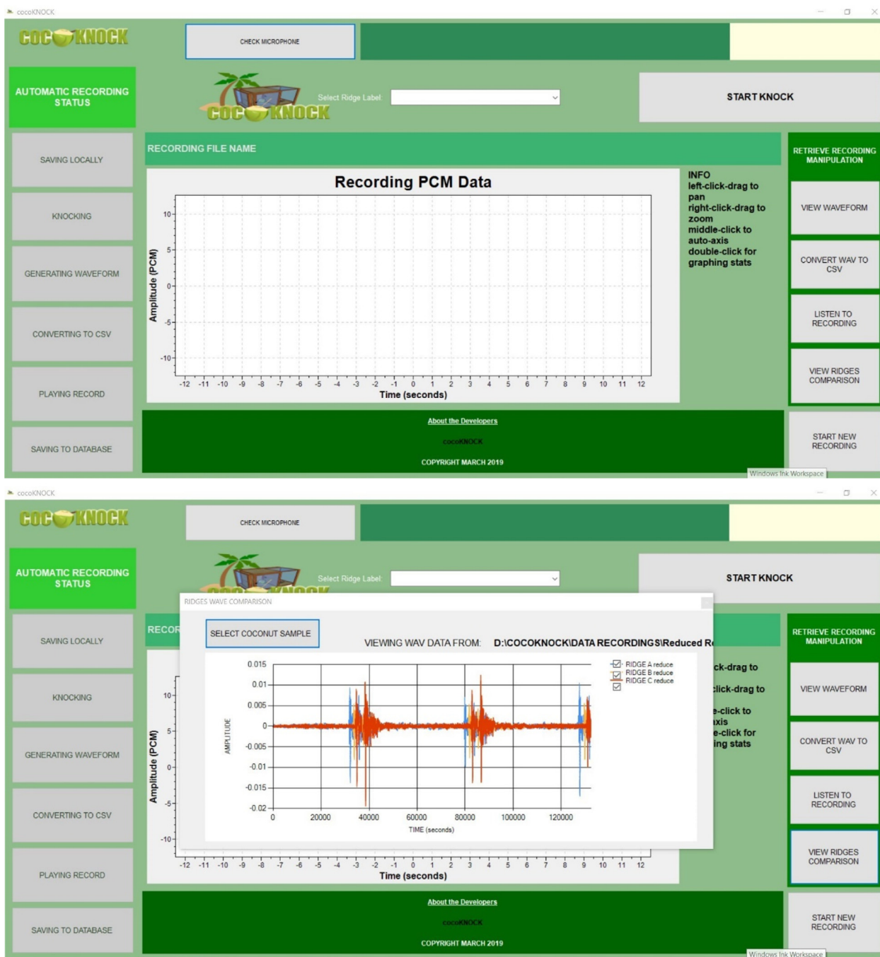
Fig. 3. CocoKnock application and interface developed to record coconut’s acoustic signal.
