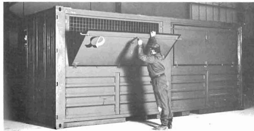
Fig. 4 Open sided container with flaps — designed by Sea Containers Ltd
