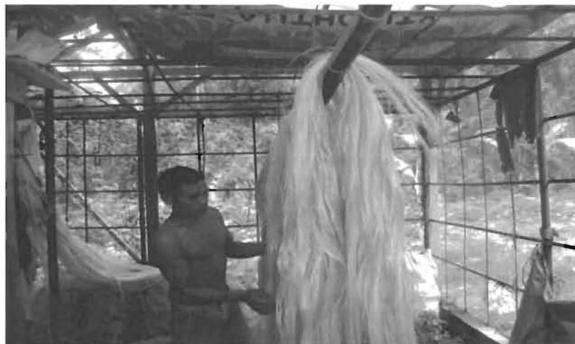
Figure 3. Drying of abaca fiber immediately after fiber extraction to avoid deterioration of fiber quality (PCA-DRC, October 2009)
