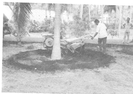
Fig. 3. Power Tiller operated basin opener with cage wheels under operation.
