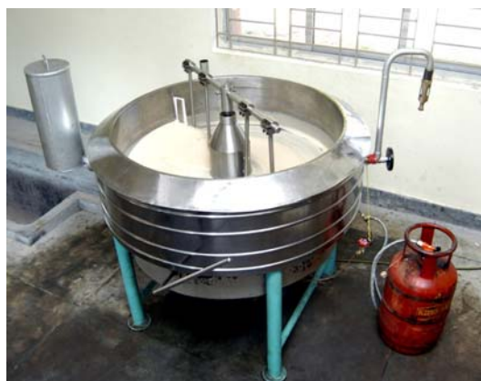
Fig. 3. Working of newly developed VCO cooker
