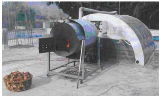
Fig.9. CPCRI Solar cum electrical dryer with agri waste as third source of energy
