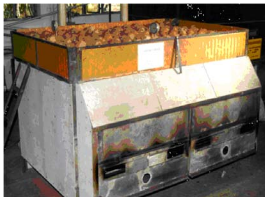
Fig.10. CPCRI Copra drier with coconut shell as fuel
