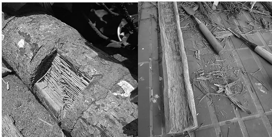
Figure 3. (a) External xylem and an inner strip of the vascular bundle and (b) cross-section after the trunk was quartered and the vascular bundle was removed.
