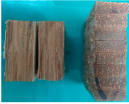
Figure 4. Glued stacked areca wood blocks. The cracked section within the block indicates high adhesive strength (Chao and Lin 2019).
