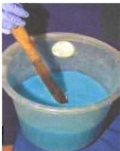
Checking of Bordeaux mixture with a knife
