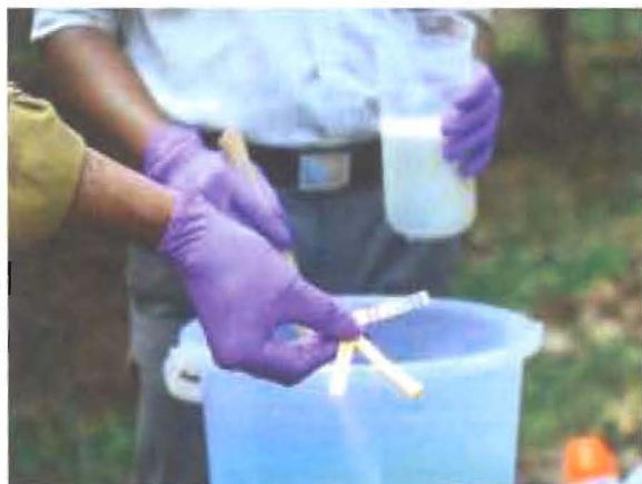
Checking the pH of the Bordeaux mixture
