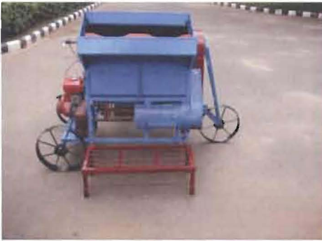
Fig. 3.25: Hold on type arecanut stripper
