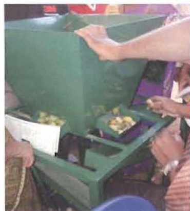
Fig. 3.29: Tender arecanut dehusking machine developed by UAS, GKVK, Bengaluru
