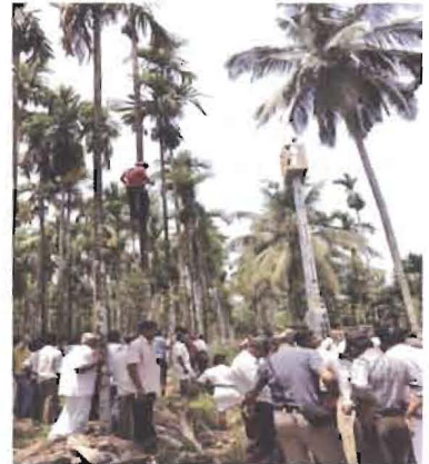
Fig. 3.21: Skylift platform mounted on tempo
