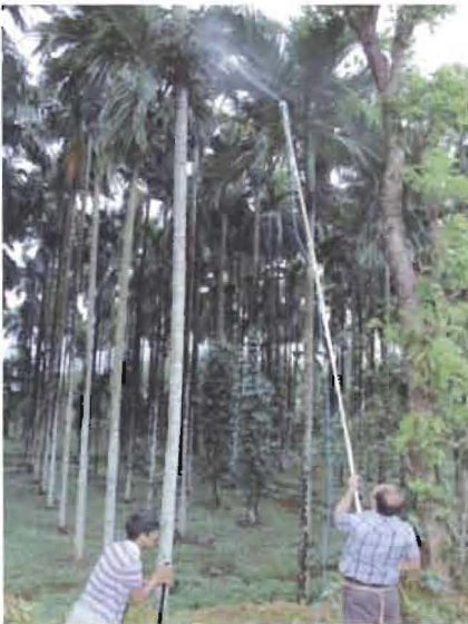
Fig. 3.9: The telescopic spray lances in operation
