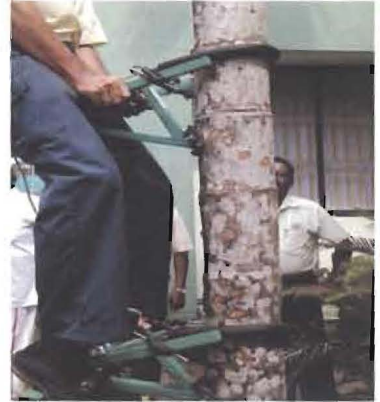
Fig. 3.20: Climbing device developed by CAMPCO Ltd and its demonstration
