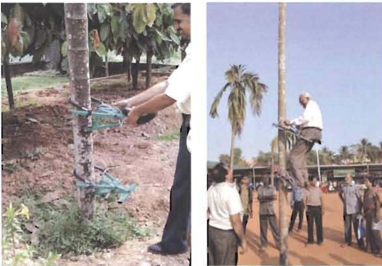
Fig. 3.19: Demonstration of the climbing device-R Tech Agri-Equipment
