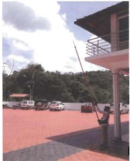
Fig. 3.10: Telescopic spray lance developed by the Redbee Engineering
