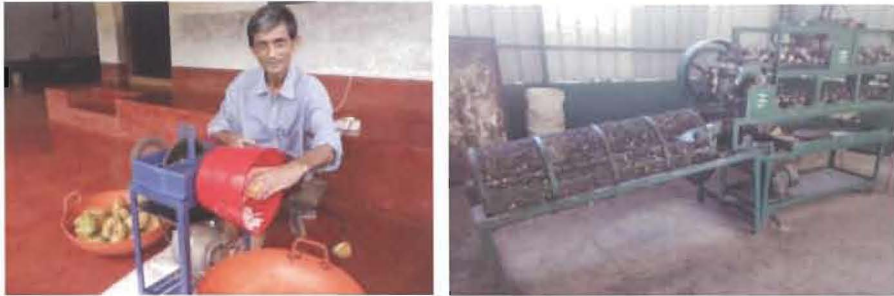
Fig. 3.35: Cocoa pod breaker- Hand operated and motorized
