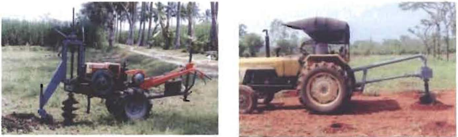
Fig. 3.2: Power tiller operated and tractor operated auger digger
