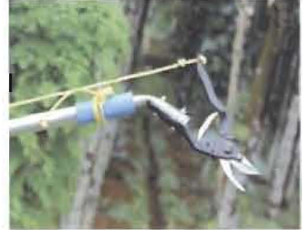
Fig. 3.32: Cocoa scion cutter device
