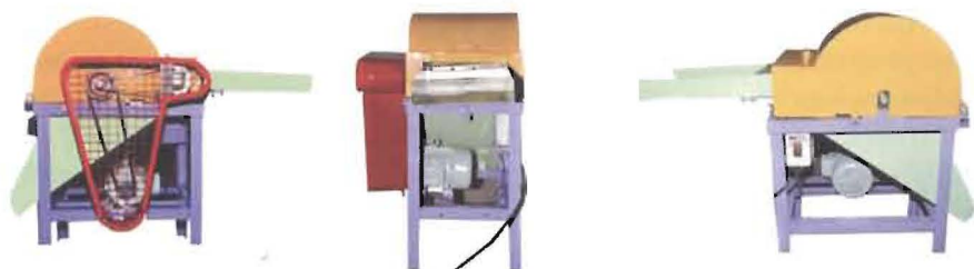
Fig. 3.30: Arecanut sheath size reduction equipment - ICAR CIAE model
