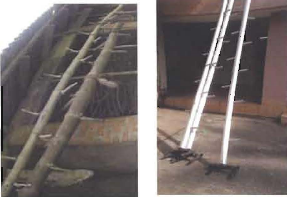
Fig. 3.16: Harvesting pole – bamboo and metallic
